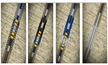
One of the benefits of washing the perforations with the Barricade system is that the standpipe pressure is a key performance indicator. High pressure indicates a high amount of debris on the back side of the casing; low pressure indicates a low amount of debris on the back side of the casing.
