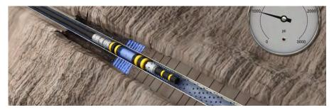
The first step of the operation was to run a Cement Bond Log to determine the optimum area to place the two barriers based on the Stronghold Barricade Systems operational window. The well was then perforated and the washing operations could commence.
