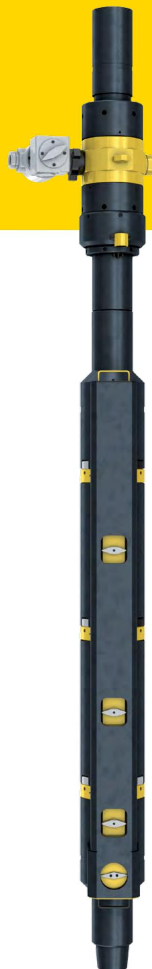
Designed to the highest standards of safety, consistency and reliability, Archer's Remote Controlled Cement Head (RCCH) allows the controlled release of setting balls and drillpipe darts without the need to stop circulation or rotation, or break connections.
