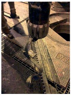
Fig 1. Clamp recovered on the circulating magnet.
