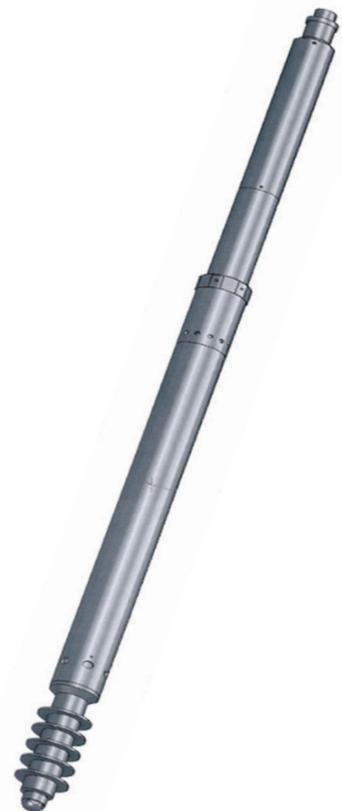
TASK/Launcher for tubing retrievable safety valves (TRSV's) utilizes the No-Go and seal areas within the TRSV normally used for an insert valve. When deployed, it lands in the No-Go profile and rubber discs fit and seal in the lower seal-bore below the flapper. This keeps TASK in place whilst it dissolves the scale in the valve.
