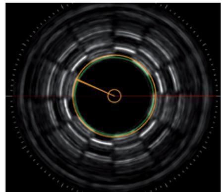
Real-time Image and measurements from **SPACE® Panorama** Survey. Green circle indicates the minimum ID of the fingers - 3.36 in. Orange circle indicates the OD of the pulling tool - 3.53 in
