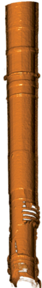
3-D rendering of SPACE® Panorama data from the entire DHSV assembly, showing damage to the flowtube while confirming dimensions and condition of seal bores and profiles.
