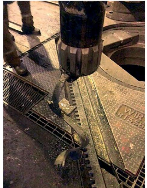
Fig 1. Clamp recovered on the circulating magnet.
